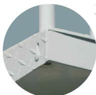
All Salter spiral stairs come with a unique design feature that provides extra strength and rigidity. Each leading baluster is locked to the front corner of the upper tread and the back corner of a lower tread. To secure the balusters to the tread we make precision pockets on the corners of each tread.
